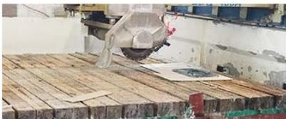
⑦ Trimming/Front Edges/Bevelling
