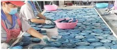
④ Splicing With Glue & Resin
